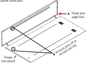
**4.** Attach the right side (Ref. No. 3) to the back in the same manner as in step 3, again making sure that the flange is around the back and that the lances on the shelf adjustment strips are pointed in the same direction as those on the back and left side.
