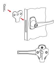
**3.** With the handle still in the open position, hook the locking bars (Ref. No. 10) to the locking cam (see "A" at left). Once in position, slowly rotate the door handle to the closed position so the lock bars prot rude from the holes at the top and bottom
