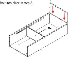
**7.** With both doors in the closed position, lift the door and frame assembly (Ref. No. 6) and place it over the cabinet body. Be aware that the door latches have not
