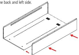
**5.** Place the shelf (Ref. No. 4) into one of the upper positions on the unit by inserting the shelf edges into the lances on all four shelf adjustment strips. Be sure that the channeled edge of the shelf is toward the cabinet front.
