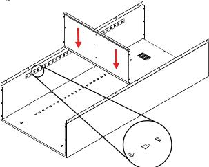
**6.** Place the top (Ref. No. 5) onto the unit. Be sure that the flanges tuck inside the cabinet sides and back. Secure with eleven nuts and bolts. The front part of the top will halt into place in step 8
